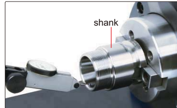
measure radial runout of shank
